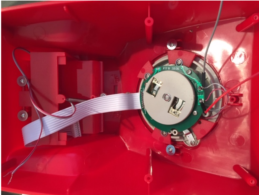
FIGURE 1. The dialer mechanism of my GPO746 with two leads soldered to the terminals of the micro-switch.
