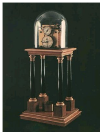
(b) Hipp Chrono- scope (1848 –) Swiss instrument widely used in early experimental psychology experi- ments on reaction times.
